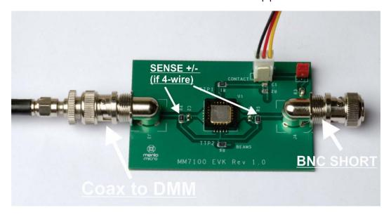
One the other hand, it is also possible to measure DC resistance using a multimeter by placing the probes on the input and output traces, next to the device, as shown in the picture below. If you zero out the multimeter test leads, you will get a good direct reading of the devices DC resistance, just a tiny bit on the high side of the correct value. R3 & R4 are also a good place to attach the SENSE lines for a 4-wire resistance measurement.
