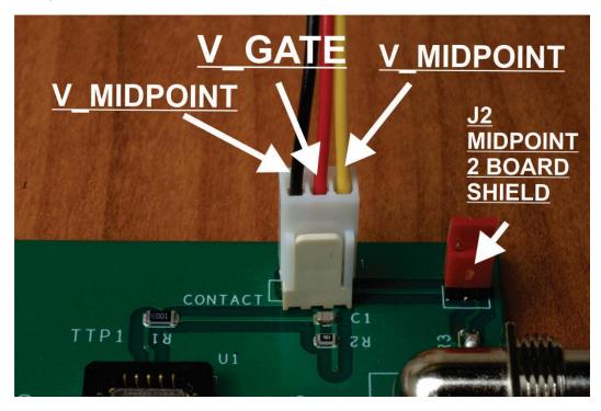
It is a good practice to monitor the current flowing into the GATE pin (J1-2) on the board. It is determined by the 10 M $\Omega$  resistor (R2) in parallel with the pin. Therefore, you should see 7.8 uA or close to this value, independent of whether the device is in the socket or not. This indicates that no current is flowing into the VGATE pin of the MM7100 device, showing that the device is operating properly.
