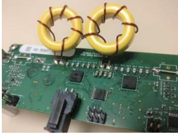
Fig. 6. MEMS-based Impedance Matching PCB
